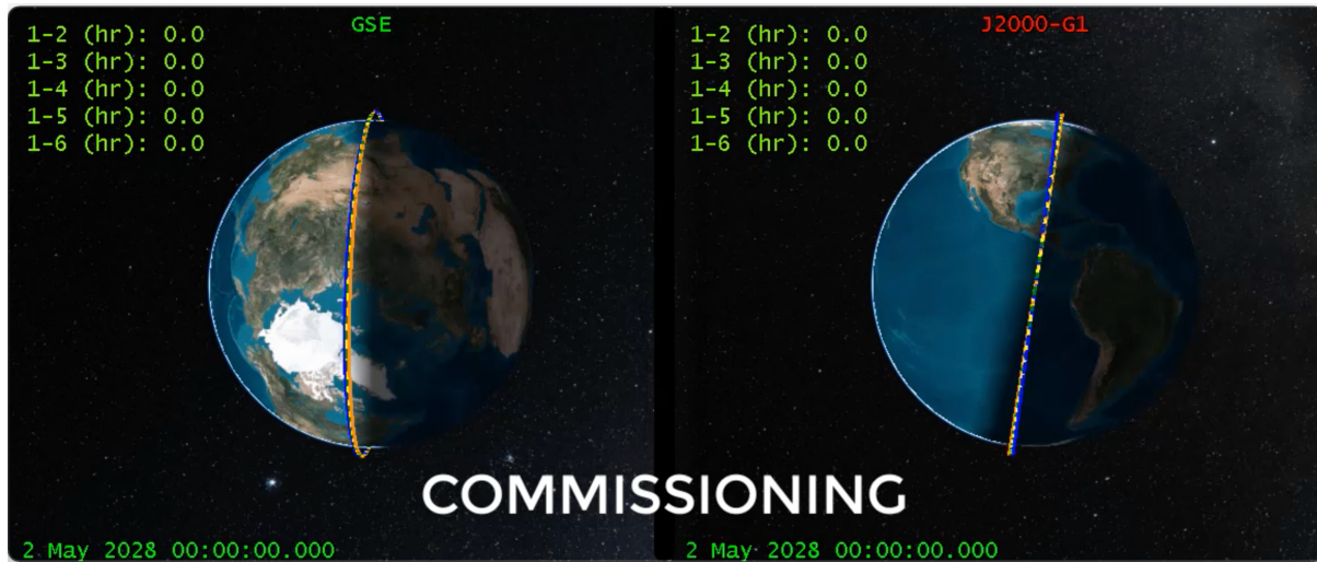
Figure 11 -- The constellation configuration at the beginning of Phase 0 (LEOC). The lines indicate orbit planes – red, orange, yellow, green, blue, violet for G1 through G6 respectively. The left view shows the view looking down onto the northern hemisphere terminator (fixed local time). The right view shows the view looking at the equator directly onto the orbit plane containing the G1 observatory. During Phase 0 the orbit planes start at the same LTAN (with slightly different inclinations). An initial launch LTAN of 1800 hours was chosen for the purposes of the DRM.
