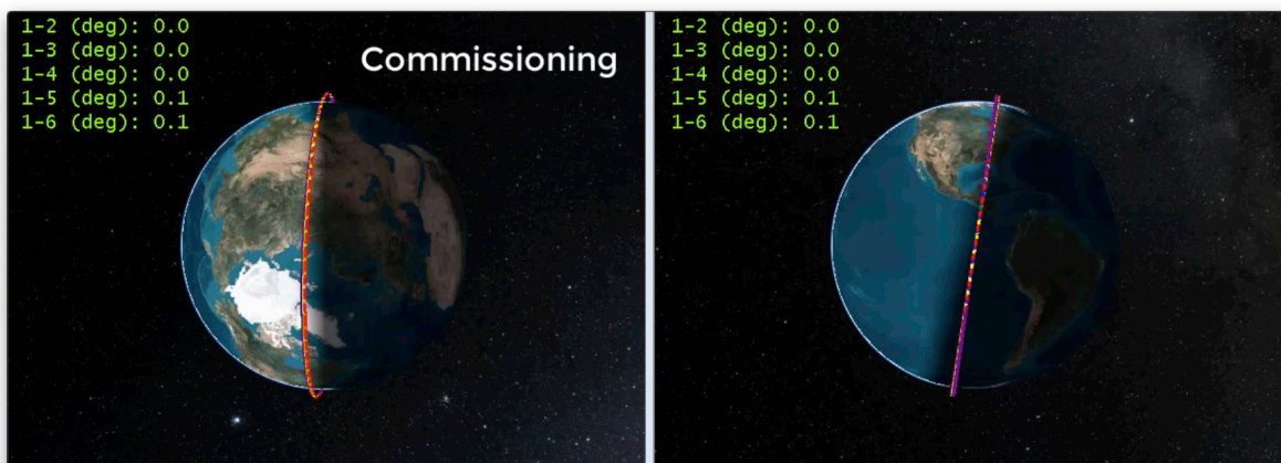
Figure 7 – The constellation configuration at the beginning of Phase 0 (LEOC). The lines indicate orbit planes – red, orange, yellow, green, blue, violet for G1 through G6 respectively. The left view shows the view looking down onto the northern hemisphere terminator (fixed local time). The right view shows the view looking at the equator directly onto the orbit plane containing the G1 observatory. During Phase 0 the orbit planes start at the same LTAN (with slightly different inclinations). An initial launch LTAN of 1800 hours was chosen for the purposes of the DRM.
