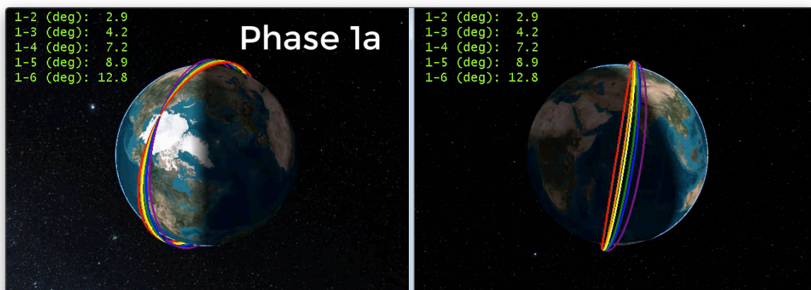
Figure 8 -- The constellation configuration at the beginning of Phase 1a (“Local-fast”), where the maximal LTAN separation between orbit planes is 12.8^\circ . The format is the same as in Figure 7.
